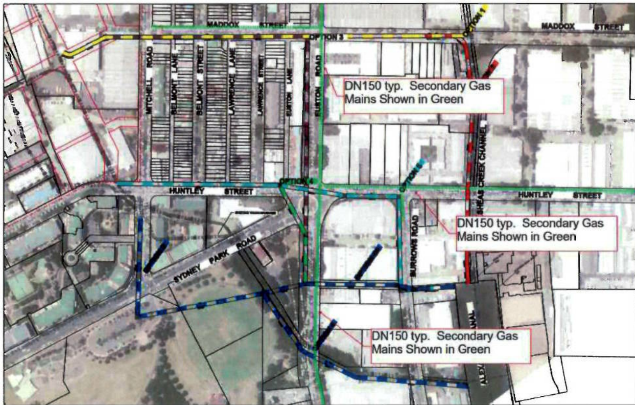
Figure 12 Jemena Secondary Gas Main Alignments
